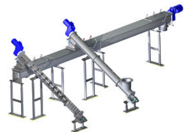
Tubular Inclined Screw Feeders Meter Bulk Materials to Horizontal U-Trough Transfer Screw Conveyor
