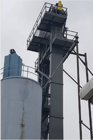
Bucket Elevators Efficiently Transport Bulk Materials Vertically
