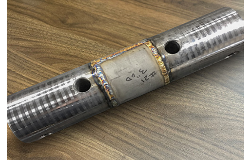
Stellite Sleeves are TIG Welded to Shaft and Finish Ground
