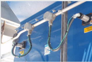
WDA Sensors Monitor Bucket Elevator Speed and Belt Alignment
