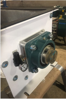
Air Regulator with Gauge Controls and Monitors Pressure
