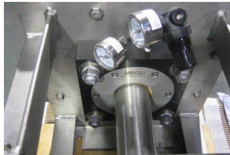
Seals are Air or Inert Gas Purged at 5 to 8-psi Above Internal Pressure of Equipment
