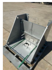
Slider Base Allows for Axial Thermal Expansion
