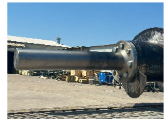
Flanged Tail Shaft is Bolted to Screw Assembly
