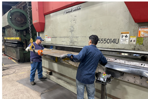
500-Ton Press is Used to Form AR-400 Trough Liners
