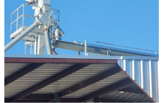
Feed is Transferred from Storage to a Bucket Elevator and then to a Transfer Screw Conveyor and Truck Load Out
