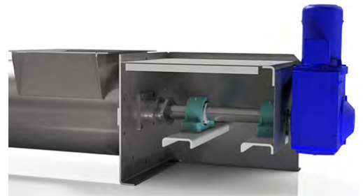
Double Bearing Arrangement Provides Rigidity and Allows for Thermal Expansion
